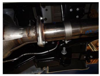
**Step 3.** Begin installation by loosely attaching the Inlet Pipe Assembly to the OEM flange outlet using the OEM hardware. Loosely attach the Extension Pipe, if needed, using the supplied clamp.
