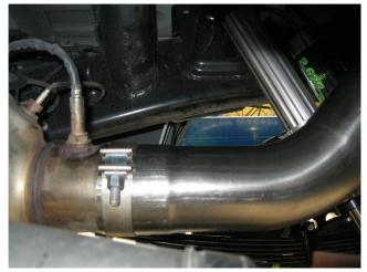
**Step 2.** Begin by attaching either the Inlet Pipe options or the Over Axle Pipe to the DPF outlet using the supplied clamp. Fit hangers into rubber insualtors on Mega Cab and Long Bed versions. Leave all clamps loose until final adjustment.
