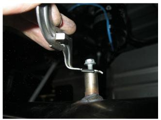
**Step 4.** When using the Long Bed extension pipe attach the OEM cable bracket using the OEM bolt.
