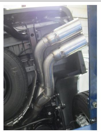
**Step 6.** Next install the Tail Pipe Assembly using the supplied 4.00" clamp and fit the welded hanger to the rubber insulator.
