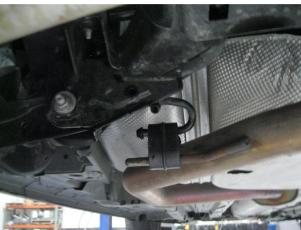
**Step 1.** To remove the OEM exhaust system, you will first need to unbolt the resonator from the catalytic converter and disengage all welded hangers from the rubber insulators. Do not damage or discard the rubber insulators, as they will be reused to mount the new system. You can now remove the exhaust from the vehicle.
