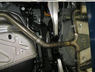
**Step 3.** Next Install the Extension Pipe Assembly to the outlet of the Resonator Assembly using a supplied 2.50" clamp, then the Y-Pipe Assembly to the Extension Pipe Assembly again using a supplied 2.50" clamp. Fit the welded hangers into the rubber insulators.
