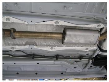
**Step 1.** To remove the OEM exhaust system, you will first need to unbolt the resonator from the catalytic converter and disengage all welded hangers from the rubber insulators. Do not damage or discard the rubber insulators, as they will be reused to mount the new system. You can now remove the OEM exhaust from the vehicle.
