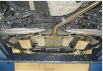
**Step 3.** Next Install the Extension Pipe Assembly to the outlet of the Resonator Assembly using the supplied 2.50" clamp. Then install the Y-Pipe Assembly to the Extension Pipe Assembly in the similar fashion using the supplied 2.50" clamp, and fitting the welded hangers into the rubber insulators.
