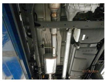
**Step 2.** Begin installation of the new system by attaching Inlet Pipe Assembly at the ball flare using the OEM clamp and fitting the hanger into the rubber insulator. Next attach the muffler to the inlet pipe using a supplied 3.50" clamp. Leave all clamps loose for final adjustment of the complete system.
