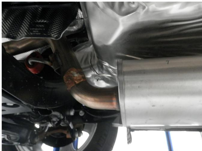
**Step 2.** You will need to cut the stock exhaust at the over axle location. Disengage hangers from rubber insulators and remove the OEM exhaust.
