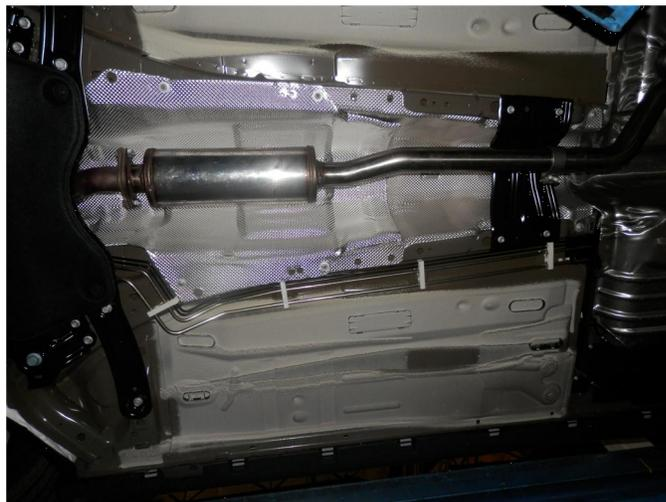
**Step 4.** Next use the supplied 2.25" clamp to loosely attach the Mid Pipe Assembly to the Inlet Muffler Assembly. Locate the welded hangers into the rubber insulators.
