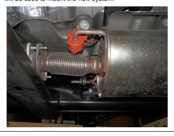
**Step 3.** Unbolt the muffler assembly from the catalytic converter outlet at the flange junction. Disengage all welded hangers from the rubber insulators. The remainder of the system can now be removed.
