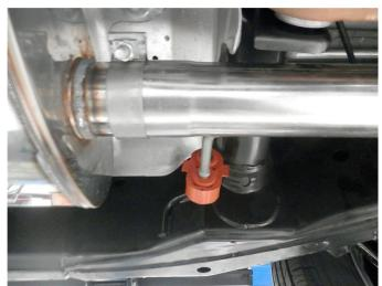
**Step 5.** Loosely attach the Over-Axle Pipe Assembly and the Tail Pipe Assembly using the supplied 3.00" clamps and engage the welded hangers to the OEM rubber insulators.
