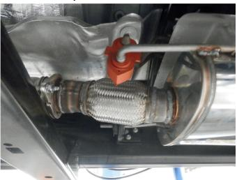
**Step 4.** Begin installing your new MAGNAFLOW system by loosely bolting the Muffler Assembly inlet flange to the OEM catalytic converter outlet using the supplied hardware.
