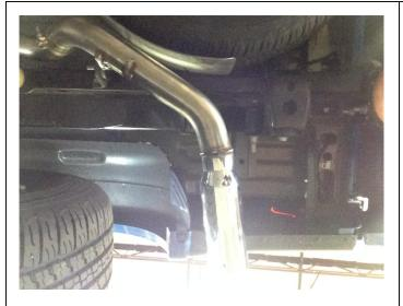
**Step 5.** Finish installing the components by sliding the Tailpipe Assembly onto the Over Axle Pipe and fastening with a supplied 3.00" Clamp. Fit the hanger into the rubber insulator.
