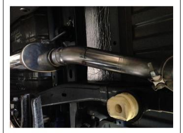
**Step 4.** Install the Over Axle Pipe using the supplied 3.00" clamps. Locate the welded hanger to the OEM rubber insulator.
