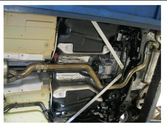
**Step 2.** Begin installation of the new system by attaching the Inlet Pipe Assembly to the factory outlet using the OEM clamp and fit the hangers into the rubber insulators. Leave all clamps loose until final adjustment.
