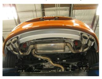
**Step 3.** Next Install the Muffler Assembly using the supplied 2.50" clamp and fit the welded hanger into the rubber insulator.
