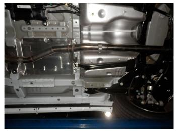
**Step 2.** Install your new system by first loosely attaching the Inlet Pipe Assembly to the catalytic converter outlet using the OEM clamp. Engage the welded hanger to the rubber insulator.
