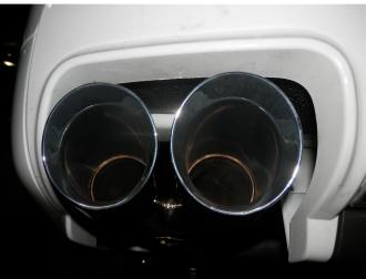
**Step 4.** Loosely install both Tail Pipe Assemblies using the supplied clamps.
