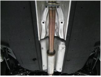
**Step 2.** Begin installation of the new system by fastening the Resonator Assembly inlet to the catalytic converter using the OEM fasteners and fitting the hanger into the rubber insulator (Leave all clamps and fasteners loose for final adjustment of the complete system.)
