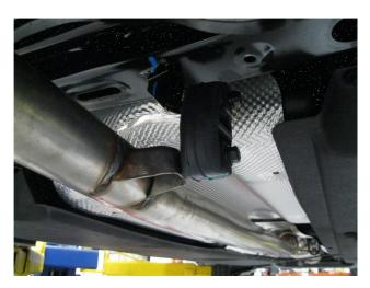
**Step 1.** To extract the OEM exhaust system begin by un-fastening the flange located behind the catalytic converter and the second flange located in front of the Driver side muffler assembly. Next, working rearward, disengage all welded hangers from the rubber insulators. Do not damage or discard the rubber insulators or fasteners as they will be re-used to mount the new system. You can now remove the exhaust from the vehicle.
