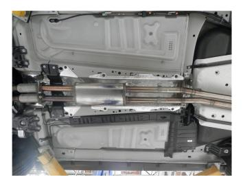
**Step 2.** Begin installation of the new system by loosely attaching the Resonator Assembly to the outlet flanges of the OE system re-using the fasteners and gasket. Fit the hangers into the rubber insulators.
