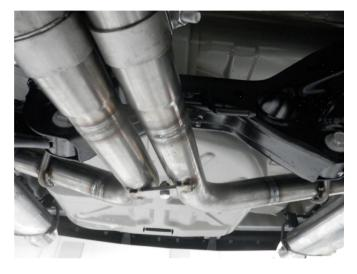
Step 4. Attach the Rear Pipe Assemblies to the Mid Pipes with the supplied 2.25" Clamps. Align the brackets and attach with the supplied fasteners and fit the hangers into rubber insulators.
