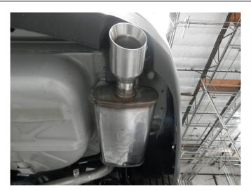
Step 5. Attach the Muffler Assemblies to the Rear Pipes with the supplied 2.25" clamps. Center the tips into the openings in the rear valance and fit the hangers into rubber insulators.
