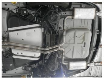
Step 3. Loosely attach the Mid-Pipe Assemblies to the Resonator Assembly with supplied 2.25" Clamps and fit the hanger into the rubber insulator.
