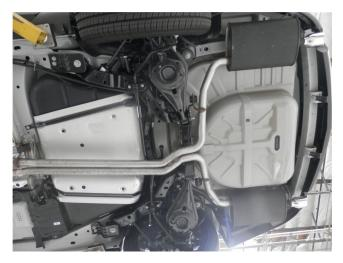
**Step 1.** Begin the removal of the OEM system by unbolting the flange at the flex joint location. Next, working rearwards (with the exhaust supported), extract the hangers from the rubber insulators and remove the OEM exhaust. Do not discard or damage the rubber insulators, flange fasteners or gasket as they will be used to install the new exhaust system.
