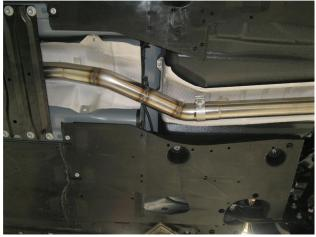
**Step 3.** Next attach the Resonator Assembly to the outlet of the catalytic converter using the supplied 2.50" Clamp followed by the Mid-Pipe using a 2.50" clamp. Leave all clamps loose until final adjustment
