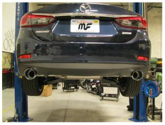
**Step 5.** Once a final position has been chosen for the new exhaust system, evenly tighten all clamps from front to rear using the torque specifications on page one of the instructions. Replace the shield and cross brace. Inspect all fasteners after 25-50 miles of operation and re-tighten if necessary.
