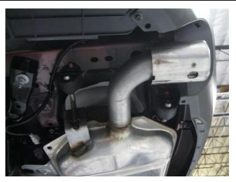
**Step 2.** Next, unbolt the flange at the muffler assembly inlet, disengage the hangers from the rubber insulators (save the rubber insulators as they will be used to install the new system) and remove the OEM system.
