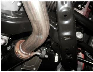
**Step 3.** Begin installation by attaching the Resonator Assembly to the outlet of the cut pipe using the supplied 2.18" Clamp and fitting the hanger into the rubber insulator. Leave all clamps loose until final adjustment
