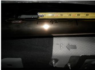
**Step 1.** Removal of the exhaust system requires cutting and de-burring the pipe 4.50" behind the welded on rear heat shield. To accomplish this you must remove the cross brace..
