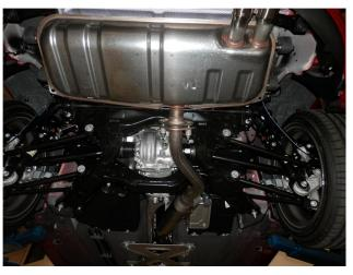
**Step 2.** Next, unbolt the flange at the muffler assemblly inlet, disengage the hangers from the rubber insulators (save the rubber insulators as they will be used to install the new system) and remove the OEM system.
