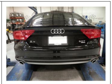
**Step 3.** Next Install the Muffler Assemblies to the outlets of the Resonator Assembly using the supplied 2.50" clamps. Insert hangers into rubber insulators.
