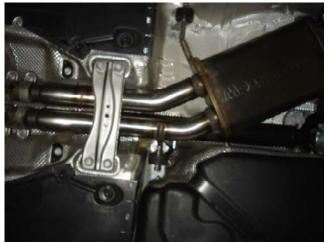
**Step 2.** Begin installation of the new system by fastening the Resonator Assembly inlet to the catalytic converter using the OEM clamps and fitting the hangers into the rubber insulators (Leave all clamps and fasteners loose for final adjustment of the complete system.)
