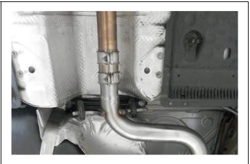
**Step 2.** Begin installation of the new system by fastening the Inlet pipe Assembly to the catalytic converter using the OEM clamp and fitting the hangers into the rubber insulators (Leave all clamps and fasteners loose for final adjustment of the complete system.)
