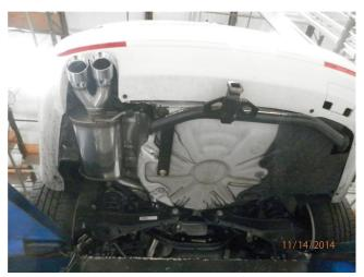
**Step 3.** Next Install the Muffler Assembly to the inlet Pipe Assembly using the supplied 2.50" clamp. Insert the hanger into rubber insulator.
