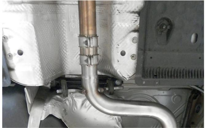
**Step 2.** Begin installation of the new system by fastening the Inlet pipe Assembly to the catalytic converter using the OEM clamp and fitting the hangers into the rubber insulators (Leave all clamps and fasteners loose for final adjustment of the complete system.)
