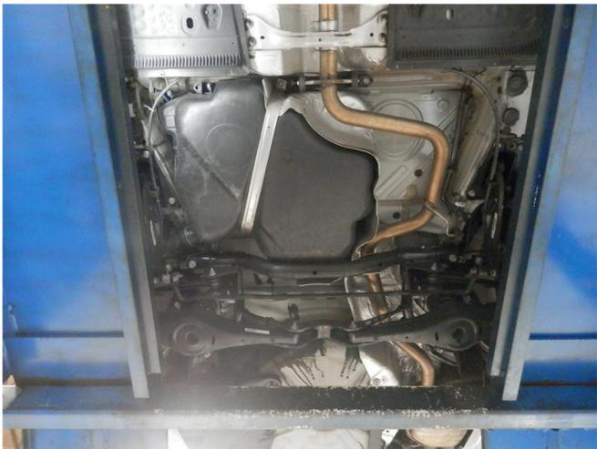
**Step 1.** To remove the OEM exhaust system you will need to cut it into two pieces just above the rear sway bar. Once the exhaust is cut you can begin removing it by loosening the clamp located behind the catalytic converter (just above the cross brace). Working rearward, disengage all welded hangers from the rubber insulators. Do not damage or discard the rubber insulators or fasteners as they will be re-used to mount the new system. You can now remove the exhaust from the vehicle.
