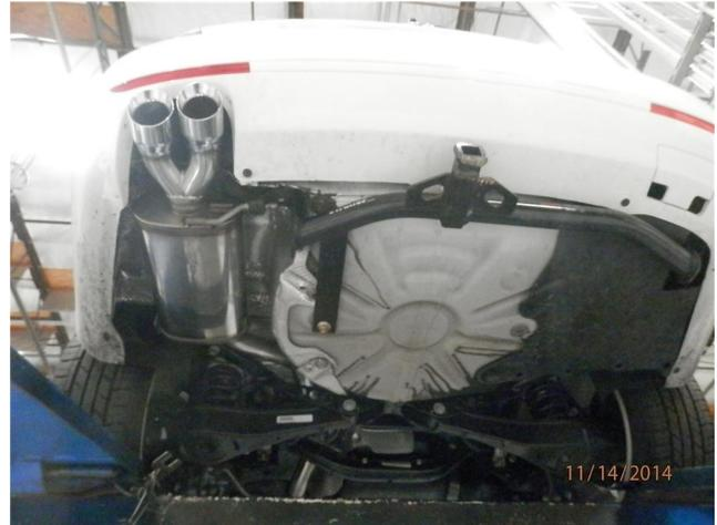
**Step 3.** Next Install the Muffler Assembly to the inlet Pipe Assembly using the supplied 2.50" clamp. Insert the hanger into rubber insulator.
