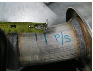
**Step 2.** Begin removing the OEM exhaust system by cutting both pipes going into the muffler assemblies. Measure and cut 2.0" driver side, 1.75" Passenger side, behind the exhaust valve welds as shown. Next extract the hangers from the rubber insulators and remove the OEM mufflers. Retain rubber insulators and as they will be used to install the new system.
