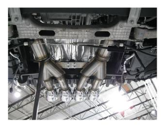
**Step 3.** Begin installation of the new system by attaching the passenger side Muffler Assembly first using the supplied 2.50" clamp. This is important for connecting bracket orientation (driver side on bottom). Install the driver side Muffler Assembly with the supplied clamp and attach brackets using the supplied fasteners as shown. Keep clamps and fasteners loose until final positioning. Finish by installing rear valance
