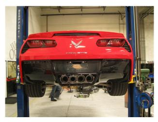
**Step 4.** Once a final position has been chosen for the new exhaust system, evenly tighten all clamps from front to rear using the torque specifications on page one of the instructions. Inspect all clamps and fasteners after 25-50 miles of operation and re-tighten if necessary.
