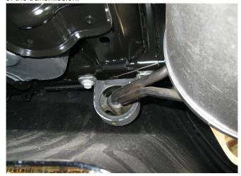
**Step 5.** Unbolt both hanger brackets located either side of the muffler assemblies. Unclip the plug connecting the valve motor assemblies to the inlet pipes. Disconnect the wiring harness on both sides of the tail pipe assemblies.
