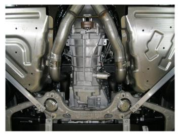
**Step 7.** Begin installation of you new MAGNAFLOW exhaust system by attaching each valve motor to the new system using the OEM fasteners. Install both drivers side and passengers side Inlet Pipe Assemblies to the OEM X-Pipe. Loosely secure using the OEM clamps.
