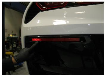
**Step 1.** To remove the OEM exhaust system you will first need to remove the rear valance. To do so you will need to remove The two 10mm bolts behind each reflector, the two 10mm bolts behind the license plate and two more 10mm bolts just underneath the license plate.
