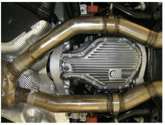
**Step 3.** Install the new system by loosely securing the D/S and P/S inlet pipes to the outlet pipes you have just cut using the supplied 2.50" clamps. Leave all clamps and fasteners loose for final adjustment of the complete system once installed.
