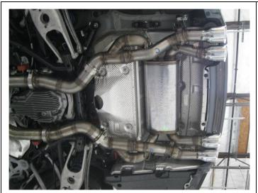
**Step 5.** Attach both OEM exhaust control valve motors to the valve brackets on the new system locating the motor shaft to the valve bushing. You may now install the Muffler Assembly using the same procedure for the V-Band Clamps. Engage the hanger bracket using the OEM hardware.
