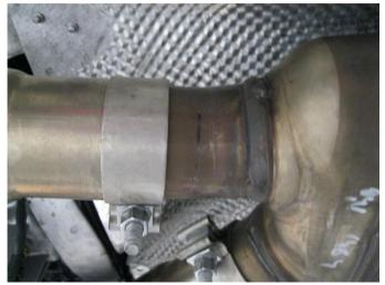
**Step 2.** You will need to cut the two outlet pipes 4.00" rearward of the underbody muffler. Disengage all welded hangers from the OEM rubber insulators. Do not discard the OEM fasteners or damage the rubber insulators as they will be needed to mount your new MAGNAFLOW system. Once the OEM system has been removed you can unbolt the two exhaust control valves located on the muffler assembly.
