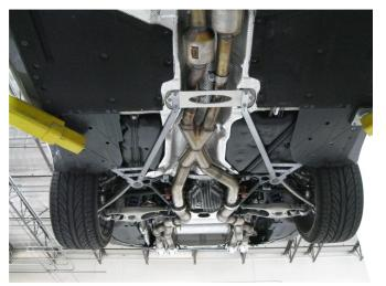
**Step 3.** Install the new system by loosely securing the inlet pipes of the X-Pipe Assembly to the outlet pipes you have just cut using the supplied 2.50" clamps. Leave all clamps and fasteners loose for final adjustment of the complete system once installed.
