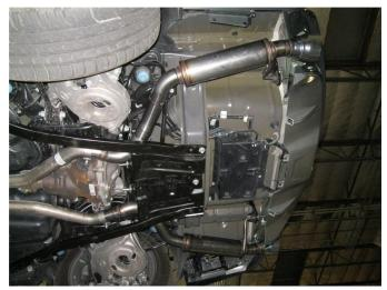
**Step 3.** Next attach both Muffler Assemblies to the Inlet Pipe Assemblies using the supplied 2.50" clamps and fitting the hangers into the rubber insualtors.
