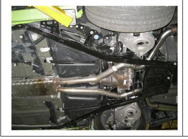
**Step 2.** Begin installation of the new system by attaching both Inlet Pipe Assemblies to the pipes you have just cut. Loosely secure using the supplied 2.25" clamps. Engage the welded hangers to the rubber insulators. Leave all clamps loose until final adjustment.
