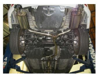
**Step 4.** Next use the supplied 2.25" clamps to attach the Muffler Assemblies to the Y-Pipe Assembly and insert the hangers into rubber insulators.
