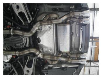
**Step 5.** Attach both OEM exhaust control valve motors to the valve brackets on the new system locating the motor shaft fo the valve bushing. You may now install the Muffler Assembly using the same procedure for the V-Band Clamp. Engage the hanger bracket using the OEM hardware.
