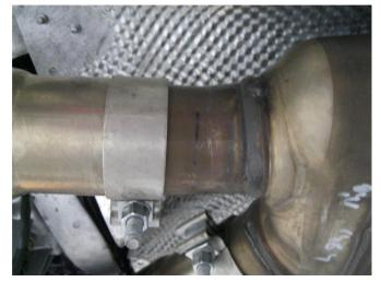
**Step 2.** To remove the OEM exhaust system you will need to cut the two outlet pipes 4.00" rearward of the underbody muffler. Disengage all welded hangers from the OEM rubber insulators. Do not discard the OEM fasteners or damage the rubber insulators as they will be needed to mount your new MAGNAFLOW system. Once the system has been removed you can unbolt the two exhaust control valve motors located on the valve bracket on the muffler assembly.
