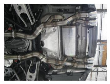
**Step 5.** Attach both OEM exhaust control valve motors to the valve brackets on the new system locating the motor shaft to the valve bushing. You may now Install the Muffler Assembly using the same procedure for the V-Band Clamp. Engage the hanger bracket using the OEM hardware.
