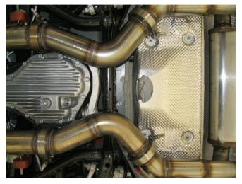
**Step 4.** Loosely Install the D/S and P/S Mid Pipe Assemblies with the supplied V-Band Clamps. \*\*NOTE: Take care when using the V-Band Clamps, they are designed for one time use only. Once the clamp is tightened it can not be reused.
