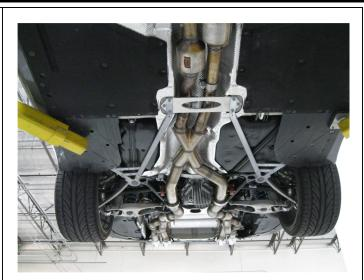
**Step 3.** Install the new system by loosely securing the inlet pipes of the X-Pipe Assembly to the outlet pipes you have just cut using the supplied 2.50" clamps. Leave all clamps and fasteners loose for final adjustment of the complete system once installed.
