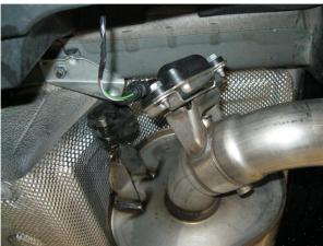
**Step 1.** To remove the OEM exhaust system you will need to remove the cross braces/stiffener and unplug the electronic exhaust control valve at the rear of the vehicle. Start by loosening the v-band clamp at the catalytic converter junction, working rearward disengage the hangers from the rubber insulators (retain rubber insulators and OEM v-band clamp) and remove the OEM system.
