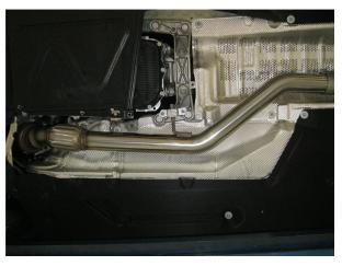
**Step 3.** Begin installation of the new system by fastening the Inlet Pipe Assembly to the outlet of the catalytic converter using the OEM v-band clamp and fitting the hanger into the rubber insulator.
