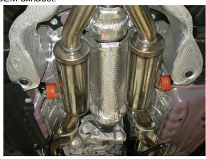
**Step 3.** Begin installation of your new MAGNAFLOW system by attaching the Driver and Passenger side Resonator Assemblies at the two bolt flange locations using the supplied 10MM bolts and the OEM nuts and springs and fitting the hangers into the rubber insulators. Keep all fasteners and clamps loose until final adjustment.
