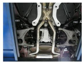
**Step 4.** Next use the supplied 2.50" clamps to attach the X-Pipe to the Resonator Assemblies.
