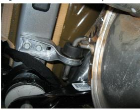
**Step 2.** Working rearward disengage the hangers from the rubber insulators and un-fasten the two bolt flange at the driver side rear muffler and remove the OEM exhaust.
