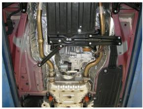
**Step 1.** Begin removal of the OEM exhaust system by unfastening the spring loaded two bolt flanges located in front of the factory resonator.
