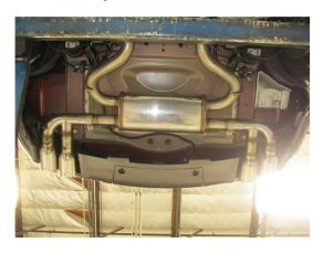
**Step 5.** Finish by attaching the Muffler Assembly to the Mid Pipe and the Tail Pipe Assemblies to the Muffler using the supplied 2.50" clamps. Fit hangers into rubber insulators.
