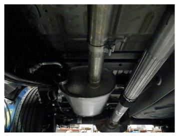
**Step 1.** The new exhaust system requires that you remove the spare tire from the vehicle. To remove the OEM exhaust system, loosen the clamp attaching the system inlet pipe to the resonator outlet pipe. Disengage all welded hangers from the OEM rubber insulators. Do not discard the OEM clamp or damage the rubber insulators as they will be needed to mount your new MAGNAFLOW system.
