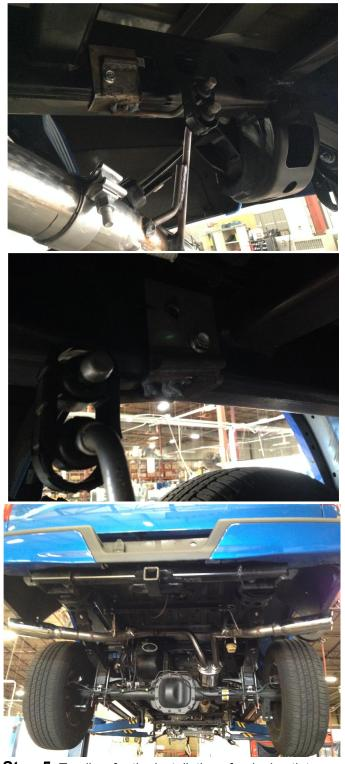
**Step 5.** To allow for the installation of a dual outlet system on a single outlet vehicle you will have to mount the supplied Hanger Brackets to existing holes in the factory frame rails using the supplied fasteners (8mm bolt and panel nut) as shown in the photos. Once completed you can now slide the Tailpipe assemblies onto the Over Axle pipes and fasten with the supplied 2.50" clamps and mount the hangers to the installed hanger brackets using the supplied rubbber insulators.
