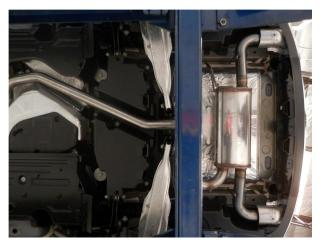
**Step 4.** Complete the installation by attaching the Muffler Assembly to the Mid-Pipe using a 2.50" clamp and fitting the hangers into the rubber insulators. Tailpipes should fit into factory outlets in rear valance.
