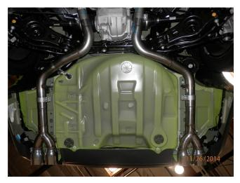
**Step 3.** At this point you have two options for tips. Magnaflow supplies a Quad tip setup that can be clamped to the Inlet Pipes and held in place with hangers and the installation is complete.
