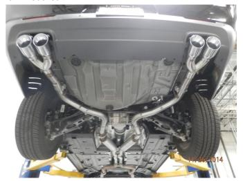
**Step 6.** Once the tips are removed install the Quad Tip Tailpipe Assemblies using the 2.50" supplied clamps. Locate both welded hangers to the rubber insulators.
