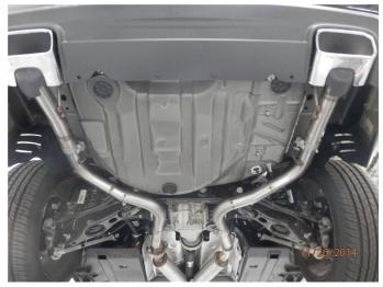
**Step 4.** To retain the OEM tips on your vehicle select the two OEM Tip Assemblies. Loosely attach each pipe inlet to the Over Axle Pipes outlets using the supplied 2.50" clamps. Engage the welded hangers for each to the rubber insulators.
