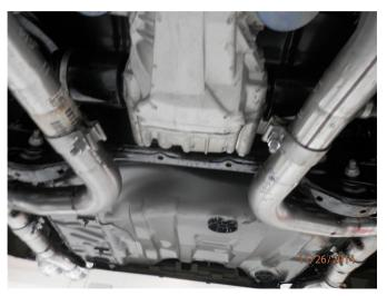
**Step 3.** Begin installation of your new system by slipping each Inlet Pipe Assembly over the cut OEM outlet pipes. Loosely secure using the supplied 2.25" clamps. Locate the welded hangers to the rubber insulators. Remember to re-attach the ground strap to the hanger. At this point you have two options for tips. Magnaflow supplies a Quad tip setup or an extension pipe assembly to allow the original OEM tips. Select the desired option before continuing the installation.
