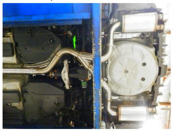
**Step 4.** Next attach the Y-Pipe Assembly to the Inlet Pipe Assembly using the supplied 3.00" clamp. Install both Muffler Assemblies in a similar fashion. Locate all welded hangers to the rubber insulators.
