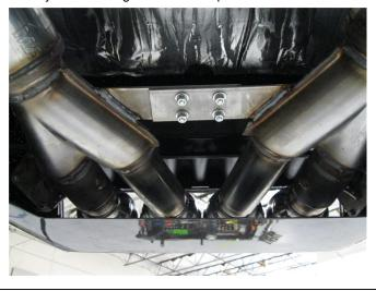
**Step 8.** Locate both OEM hanger brackets to each Tail Pipe Assembly. Next, loosely attach both assemblies to the Inlet Pipe Assembly outlets using the supplied 3.00" clamps. Using the supplied nuts, bolts and washers connect the two hanger brackets that will link both sides together. Reconnect each wiring harness connector the the valve motors. Reinstall the rear valence in the reverse order of the removal process.
