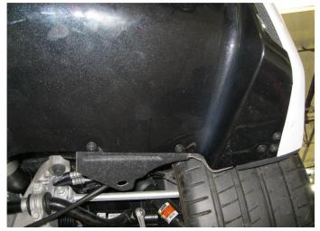
**Step 2.** Then you will need to remove the five 7mm bolts on both sides of the valance underside. Remove two 10mm bolts above the exhaust tips. The valence is fastened from the backside with molded-in plastic tabs. Release the six tabs from the valence by gently pulling each tab from the valence.
