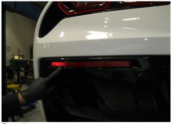
**Step 1.** To remove the OEM exhaust system you will first need to remove the rear valance. To do so you will need to remove The two 10mm bolts behind each reflector, the two 10mm bolts behind the license plate and two more 10mm bolts just underneath the license plate.
