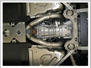
**Step 6.** Loosen both OEM clamps just rearward of the stock X-Pipe assembly. The OEM exhaust system may now be removed.
