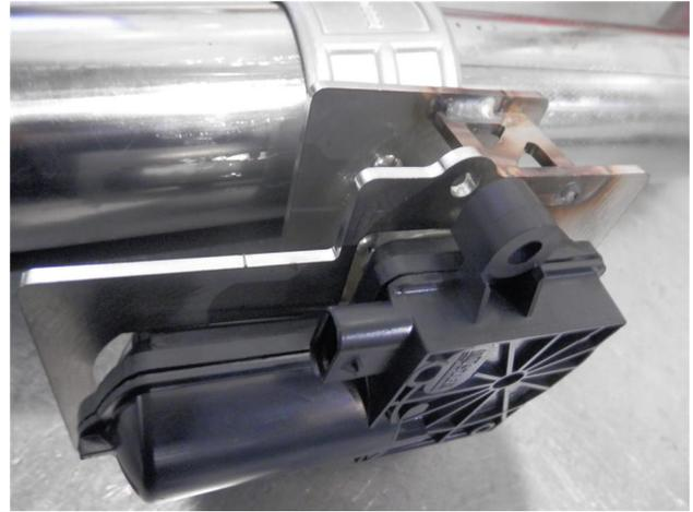
**Step 3.** With both the new and the old systems on the ground remove the valve motors from the OEM valve assemblies and mount them to the new system using the supplied hardware. The alignment spring on the motor will need to be engaged into the keyway slot of the new valve
