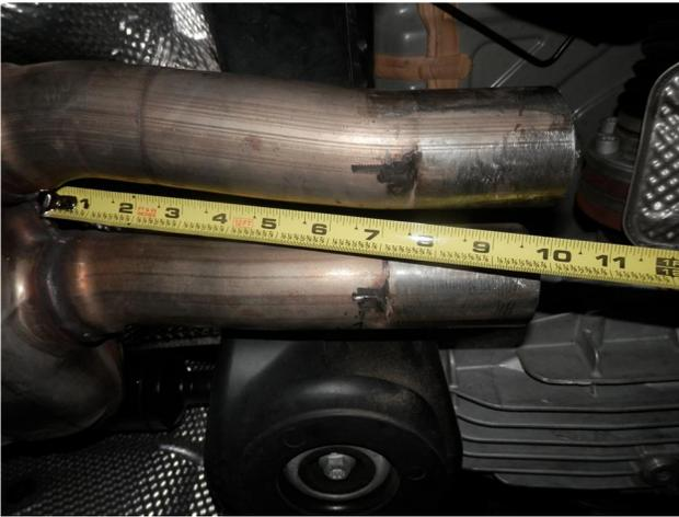
**Step 1.** Begin removing the OEM exhaust system by unplugging the electrical connectors to both rear exhaust valve motors. These motors will be re-used so care should be taken during the exhaust removal process. Next, measuring from the rear of the resonator cut both OEM pipes 10" in length.
