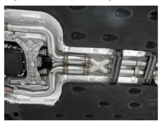
**Step 3.** Begin installation of the new Magnaflow X-Pipe by attaching the hanger assemblies to the new X-pipe while it is on the ground. Attach the X-pipe to the catalytic converter outlets using the Supplied 2.75" clamps. Fit the hanger assemblies into place and loosely fasten. Leave all hangers and clamps loose until final assembly.
