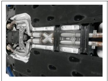
**Step 4.** Next, slip the X-pipe outlets onto the OEM inlets and fasten with the OEM clamps. Attach the rear tubing brace and both cross braces. The front tubing brace is not re-used. Once a final position has been chosen for the new exhaust system, evenly tighten all clamps from front to rear using the torque specifications on page one of the instructions. Inspect all fasteners after 25-50 miles of operation and re-tighten if necessary.
