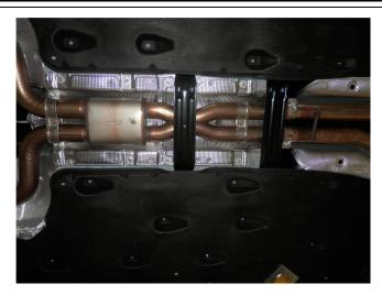
**Step 1.** Begin removal of the OEM exhaust system by detaching the two black cross braces from the underside of the vehicle and both tube braces frome the resonator assembly.
