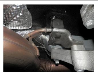
**Step 2.** Remove the OEM resonator assembly by loosening the two clamps behind each catalytic converter and the two clamps behind the X-Pipe. For ease of removal unbolt the hanger mounts from the vehicle, remove the assembly. Retain hanger assemblies, clamps and the rear tubing brace as they will be used to install the new system.
