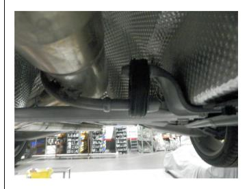
**Step 5.** Next, attach the Mid-Pipe Assembly to the Inlet pipe using the supplied 2.50" clamp and fitting the hanger to the rubber insulator.
