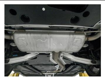
**Step 3.** With the exhaust supported, work front to rear and extract the welded hangers from the rubber insulators. Do not dicard or damage the clamp or insualtors as they will be re-used to install the new MagnaFlow exhaust.
