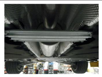
**Step 1.** To extract the OEM exhaust you will need to remove both cross braces located on the underside of the vehicle.
