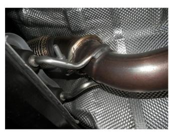
**Step 2.** Begin removing the OEM exhaust by unfastening the clamp located behind the flex pipe.
