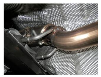
**Step 4.** Begin installation of the MagnaFlow exhaust by attaching the Inlet Pipe Assembly to the flex outlet using the factory clamp and fitting the hangers into the rubber insulators.
