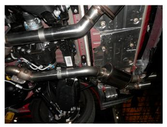
**Step 5.** Install the Muffler Assemblies to the X-Pipe Assembly with the supplied 2.75" clamps and engage the welded hangers to the rubber insulators. Leave all clamps loose for final adjustment of the system.
