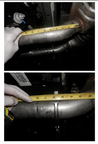
**Step 1.** It is necessary to cut the factory exhaust system to install the new Magnaflow unit. To do this measure 5.75" in front of the welds on the rear muffler inlets. Deburr the cut pipes to facilitate installation of the new system.
