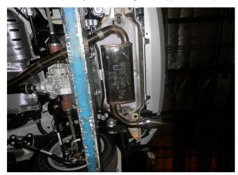
**Step 4.** Loosely install the Muffler Assembly to the Mid Pipe with the supplied clamp. Locate both welded hangers to the OEM rubber insulators.
