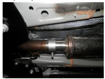
**Step 2.** Install the Resonator Assembly by slipping the inlet end over the outlet of the catalytic converter. Loosely secure using the supplied 2.18" clamp.
