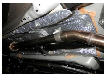
**Step 3.** Next loosely attach the Mid Pipe to the Resonator Assembly outlet using the supplied clamp.
