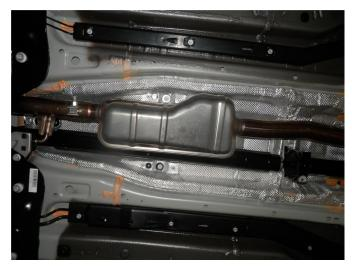
**Step 1.** To remove the OEM exhaust loosen the factory clamps in front of the resonator assembly and the one attaching the resonator assembly to the mid pipe. Disengage all welded hangers fron the rubber insulators. Be sure to retain all mounting hardware as it will be needed to install your new MAGNAFLOW system. The OEM system may now be removed.
