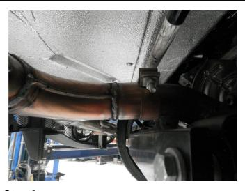
**Step 3.** Next loosely attach the Tail Pipe Assembly to the Inlet Pipe Asembly using the supplied 2.50" clamps. Engage all welded hangers to the rubber insulators.
