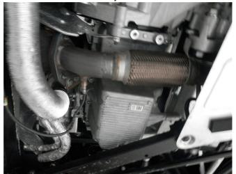
**Step 2.** Begin installation of the new system by fastening the Inlet Pipe Assembly to the catalytic converter outlet using the OEM hardware. Attach the O2 sensor. Leave all clamps loose for the final adjustment of the complete system.
