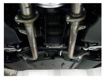
**Step 1.** Begin removal of the rear OEM exhaust mufflers by unbolting the two bolt flanges on each assembly at the resonator junction. Disengage all welded hangers from the rubber insulators. You may now remove both muffler assembles. Do not discard or damage the OEM fasteners or rubber insulators as they will be used to install the new system.
