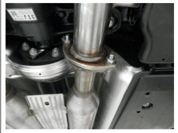
**Step 2.** To install your new MAGNAFLOW system loosely bolt each flange of the new Muffler Assemblies to the OEM resonator assemblies. Use the supplied nuts and reuse the OEM bolts.
