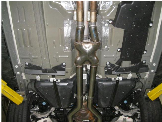
**Step 2.** Begin installation of the new system by loosely attaching the X-Pipe Assembly to the outlets using the OEM clamps. Leave all clamps loose until final adjustment.
