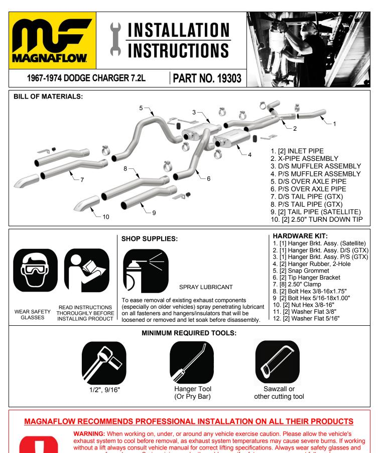
ensure a safe work area. Serious injury or death could occur if safety measures are not followed. **ATTENTION:** Always install any supplied band or U-bolt clamps to the proper torque specifications of 40-45 ft-lbs for band clamps and 30-35 ft-lbs for U-bolt clamps. Over tightening will result in the clamp breaking and
