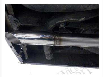
**Step 7.** Lastly, install both Polished Tips to the Tail Pipes. Once in the desired position weld each tip as shown.
