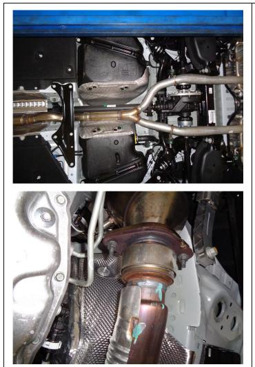
**Step 1.** To remove the OEM exhaust you will need to unbolt and remove the cross brace shown. Now you can unbolt the OEM exhaust from the catalytic converter flange junction. Disengage all welded hangers from the rubber insulators. Retain rubber insulators as they will be needed to install your new MAGNAFLOW system. The OEM system can now be removed.
