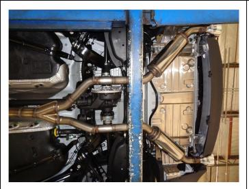
Step 4. Loosely install the drivers and passengers side Muffler Assemblies using the supplied 2.25" clamps. Engage the welded hangers to the rubber insulators.
