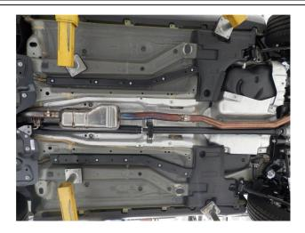
**Step 1.** To remove the OEM exhaust loosen the factory clamps in front of and behind the factory resonator assembly. Disengage all welded hangers from the rubber insulators. Retain rubber insulators as they will be needed to install your new MAGNAFLOW system. The OEM system can now be removed.
