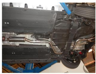
**Step 3.** Next, install the Mid Pipe Assembly, the Tail Pipe Assembly using the supplied 2.50" clamps. Locate the welded hangers to the rubber insulators.
