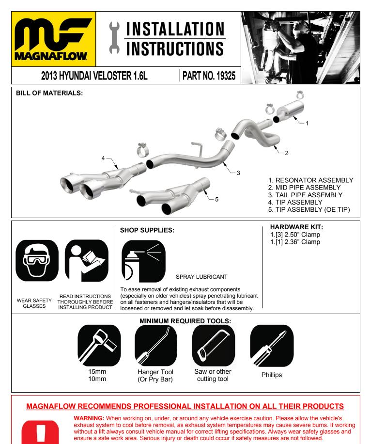
**ATTENTION:** Always install any supplied band or U-bolt clamps to the proper torque specifications of 40-45 ft-lbs for band clamps and 30-35 ft-lbs for U-bolt clamps. Over tightening will result in the clamp breaking and will NOT be warranted by MagnaFlow.
