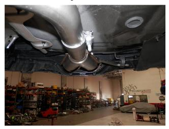
**Step 4.** The MAGNAFLOW System comes with two tip options. To retain the OEM tips locate the Tail Pipe Assembly (OE Tip) to the OEM tips. Loosely secure using the supplied 2.50" clamp. For the MAGNAFLOW tip option remove the OEM tips with the Phillips head screwdriver and 10mm socket. Now the Tail Pipe Assembly can be loosely installed using the supplied clamp locationg the welded hanger to the rubber insulator.
