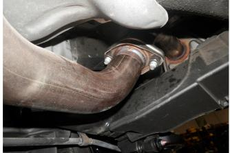
**Step 1.** To remove the OEM exhaust you will need to cut the exhaust pipe 3.00" rearward of the catalytic converter as shown. Deburr the cut edges. Unbolt the flange junction beween the OE mid pipe and muffler assembly. Disengage all welded hangers from the rubber insulators. Retain rubber insulators as they will be needed to install your new MAGNAFLOW system. The OEM system can now be removed.
