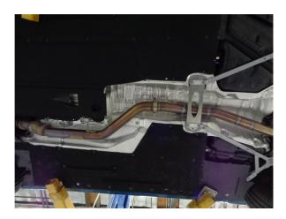
**Step 4.** Next fasten the Resonator Assembly to the inlet pipe using the supplied 3.00" clamp.
