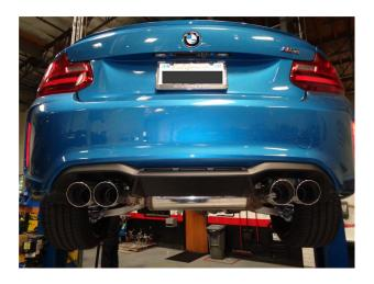
**Step 7.** Once a final position has been chosen for the new system, evenly tighten all clamps from front to rear using the torque specifications on page one of the instructions. Inspect all fasteners after 25-50 miles of operation and re-tighten if necessary.
