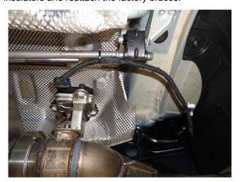
**Step 6.** To re-attach the plug to the valve motor you will need to release the loom from its mounting point on the inner body wall. Attach the connector to the valve then use one or both of the supplied Zip Ties to sucure the loom to the hanger as shown,.
