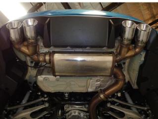
**Step 5.** Complete the installation by attaching the Extension Pipe to the Mid Pipe and the Muffler Assembly to the Extension Pipe using the supplied 3.00" clamps. Fit the hangers on the Muffler Assembly into the rubber insulators and reattach the factory braces.
