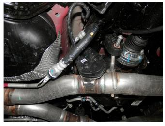
**Step 2.** Next you will need to unplug the electrical connection on the Exhaust Valve Control Motors (Qty 2) located on the OEM exhaust assembly.
