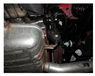
**Step 3.** Working front to rear disengage all welded hangers from the rubber insulators and remove the system. (Retain the insulators as they will be needed to mount the new MAGNAFLOW system.) Once the OEM system is on the ground transfer all the valve motors over to the new Magnaflow exhaust system.
