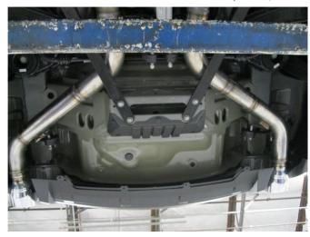
**Step 3.** Begin installation of the new system by sliding the D/S and P/S Muffler Assembly inlets onto the cut outlet of the OEM exhaust and loosely fasten with the supplied 2.75" clamps. Fit the hangers into the rubber insulators.
