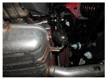
**Step 2.** Working front to rear disengage all welded hangers from the rubber insulators and remove the muffler assembly. (Retain the insulators as they will be needed to mount the new MAGNAFLOW system.)
