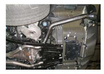
**Step 3.** Next attach both Tailpipe Assemblies to the Inlet Pipe Assemblies using the supplied 2.50" clamps and fitting the hangers into the rubber insualtors.
