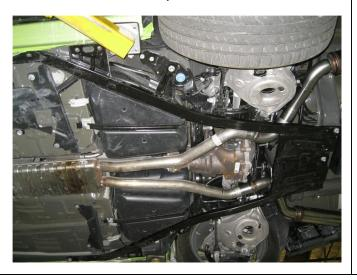
**Step 2.** Begin installation of the new system by attaching both Inlet Pipe Assemblies to the pipes you have just cut. Loosely secure using the supplied 2.25" clamps. Engage the welded hangers to the rubber insulators. Leave all clamps loose until final adjustment.
